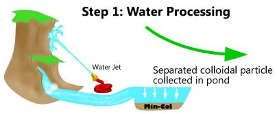
Stream of water blasts out soft rock phosphate from hard rock phosphate
